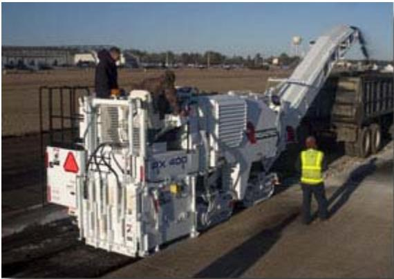
***Sample of an asphalt milling machine***
